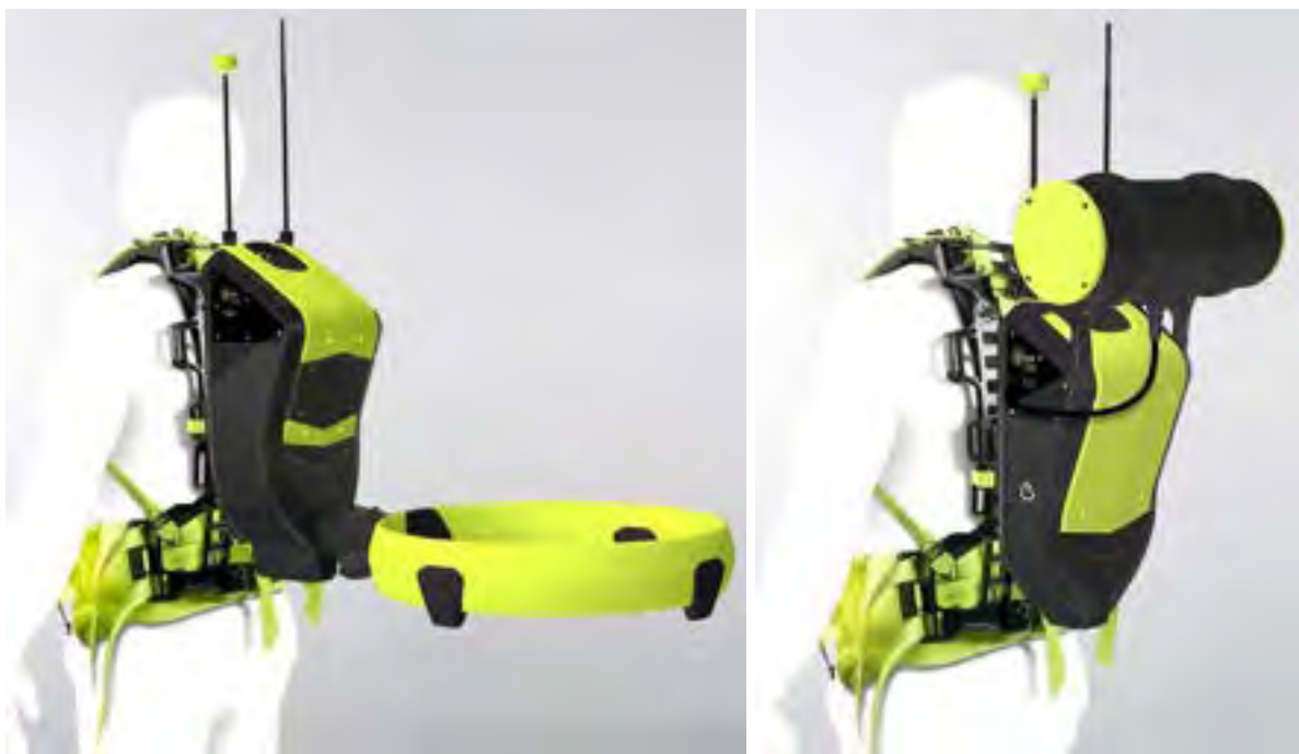
Figure 1: Illustrations of the transmitter (left) and receiver system (right) (obtained from Street et al. 2018).
